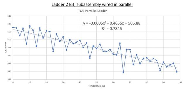
The chart above shows the TCR of the parallel circuit structure.
